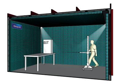
The Chronos 1F is designed to perform emission tests on automotive components. The design of the structure is optimised for maximum performances, in minimum space. The shielding and its pyramidal absorbers are manufactured by SIFPFL.
